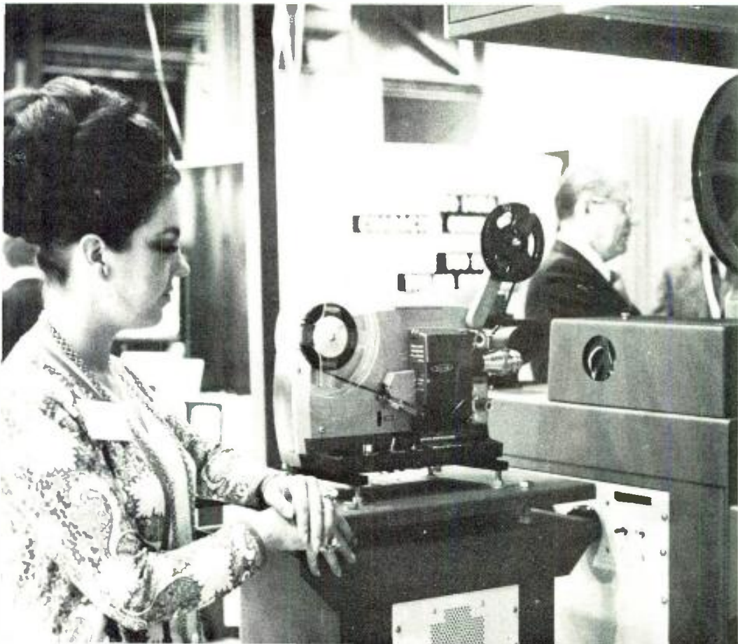
One of the new breed of telecine gear is the Wilcam Super 8 TV projector, based on a Bolex SM 8 and available through TeleMation. One version has still-frame capability for precise cueing.
