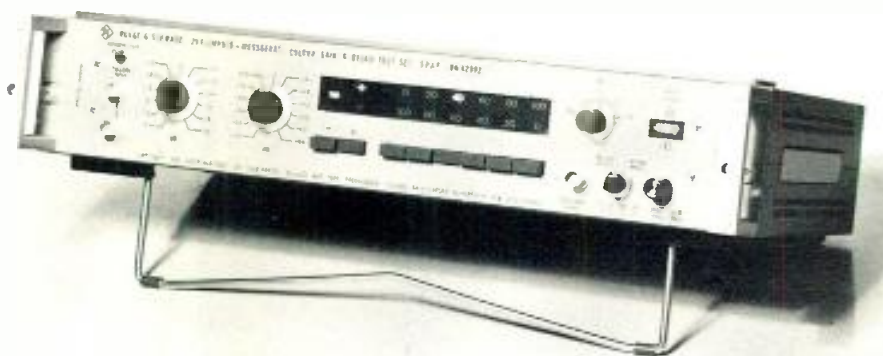
Rohde & Schwarz gain and delay test set has been modified for 12.5T pulse.
